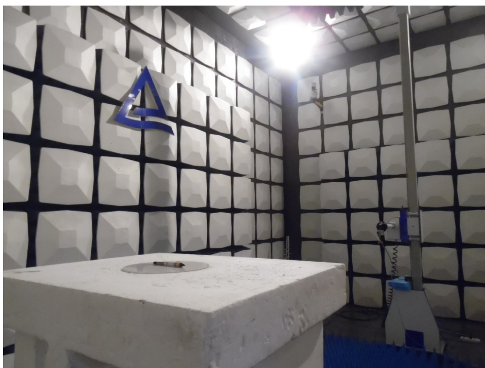
Photograph 4: Set-up for Radiated Spurious Emission, 18GHz - 26.5GHz
