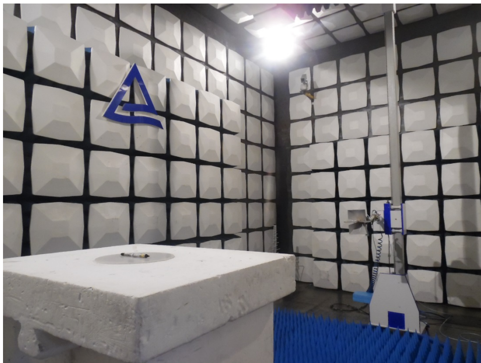
Photograph 3: Set-up for Radiated Spurious Emission, 1GHz - 18GHz
