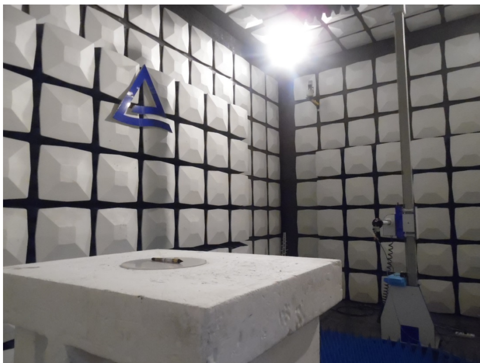
Photograph 4: Set-up for Radiated Spurious Emission, 18GHz - 26.5GHz
