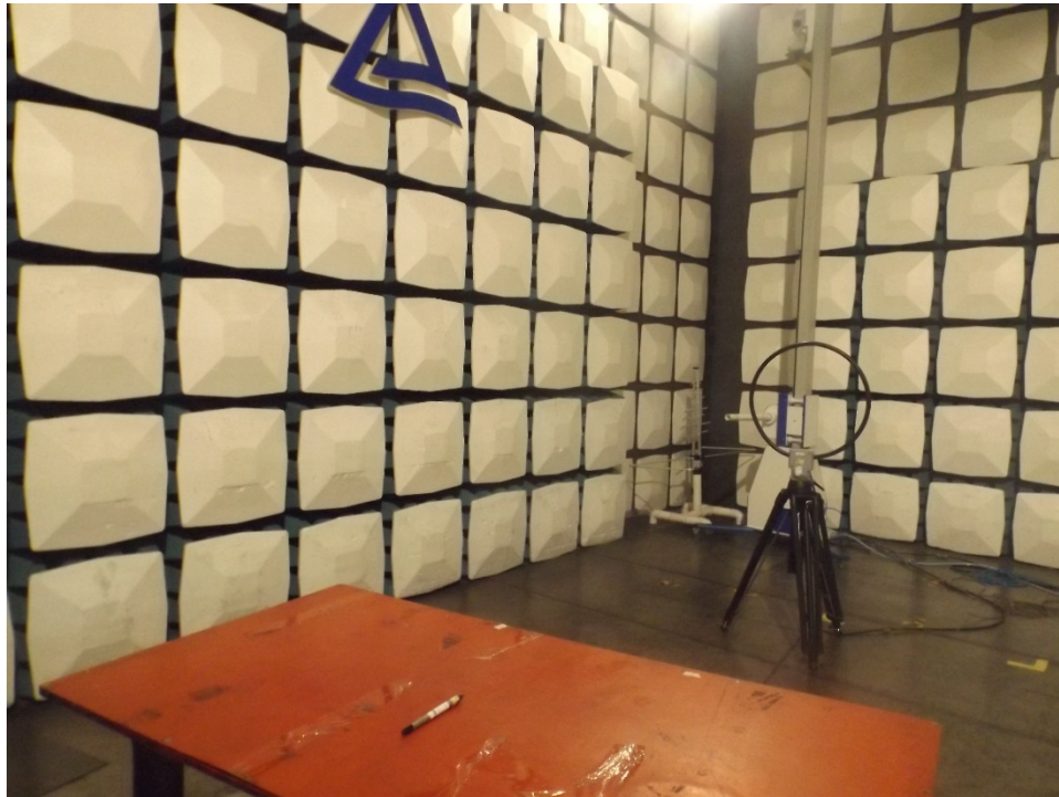
Photograph 1: Set-up for Radiated Spurious Emission, 9kHz - 30MHz
