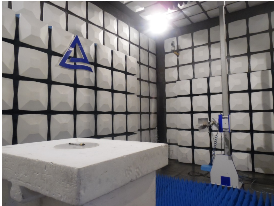
Photograph 3: Set-up for Radiated Spurious Emission, 1GHz - 18GHz
