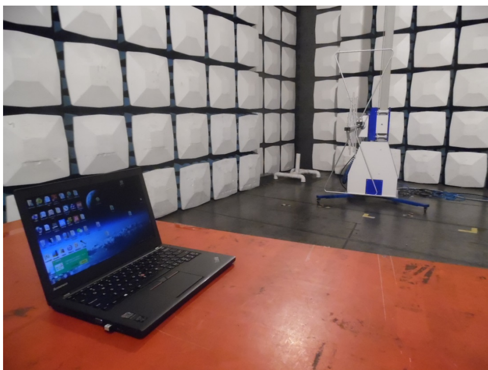
Photograph 2: Set-up for Radiated Spurious Emission, 30MHz - 1GHz
