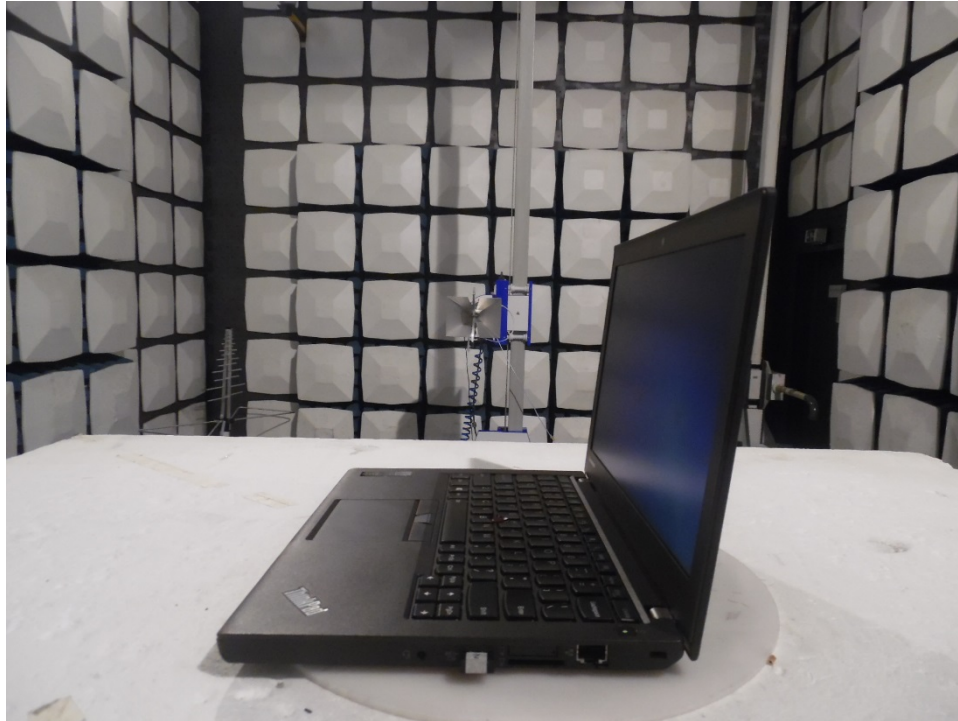
Photograph 3: Set-up for Radiated Spurious Emission, 1GHz - 18GHz
