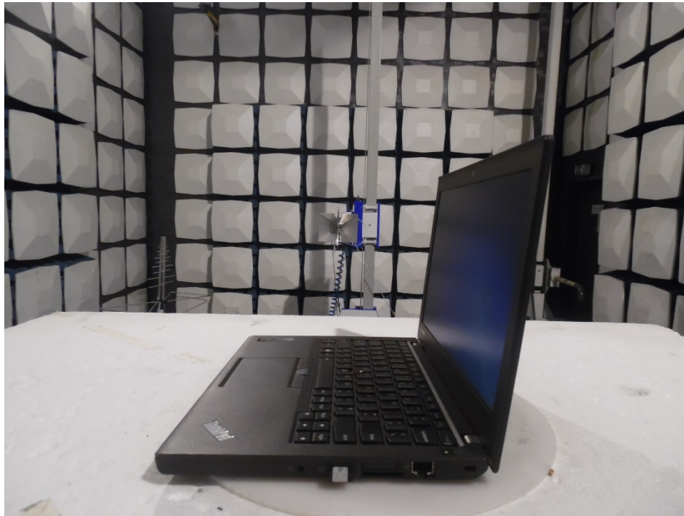
Photograph 3: Set-up for Radiated Spurious Emission, 1GHz - 18GHz
