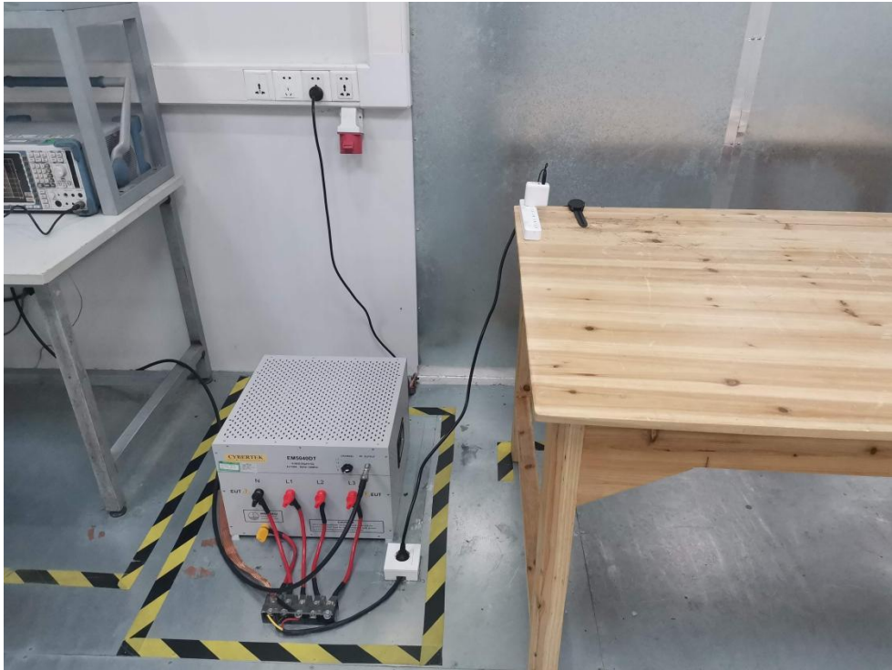
Photo of Conducted Emission Measurement
