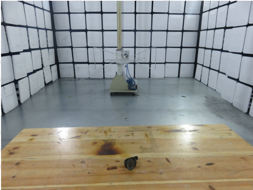
Photo of Radiation Emission Test
