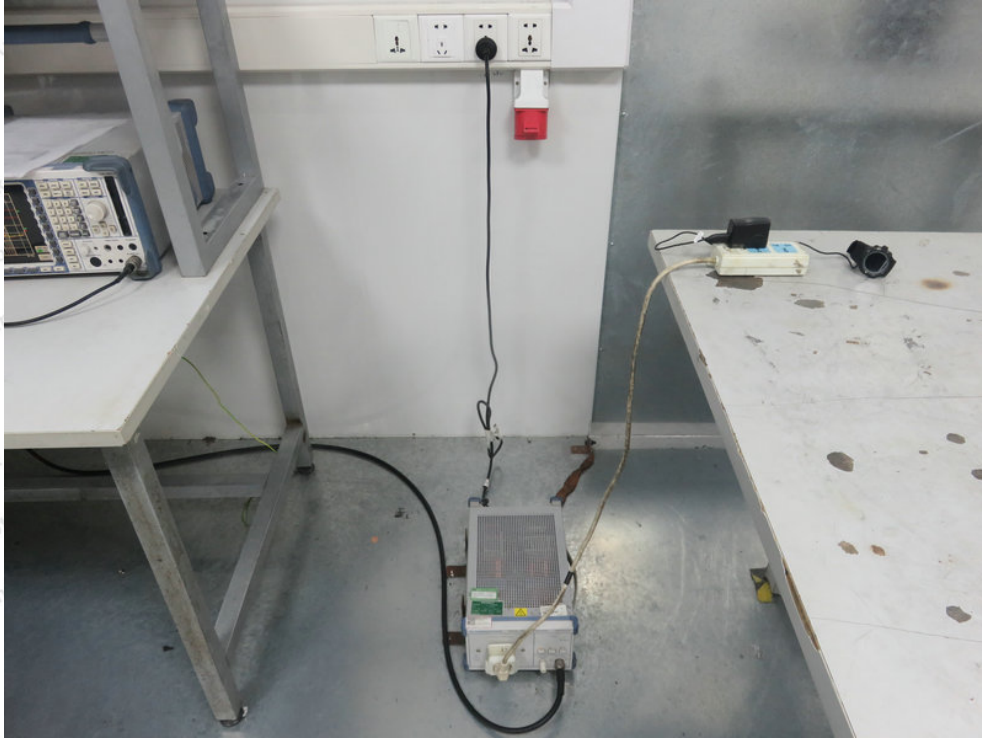
Photo of Conducted Emission Measurement
