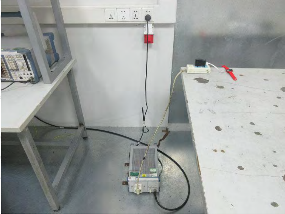
Photo of Power Line Conducted Emission Test
