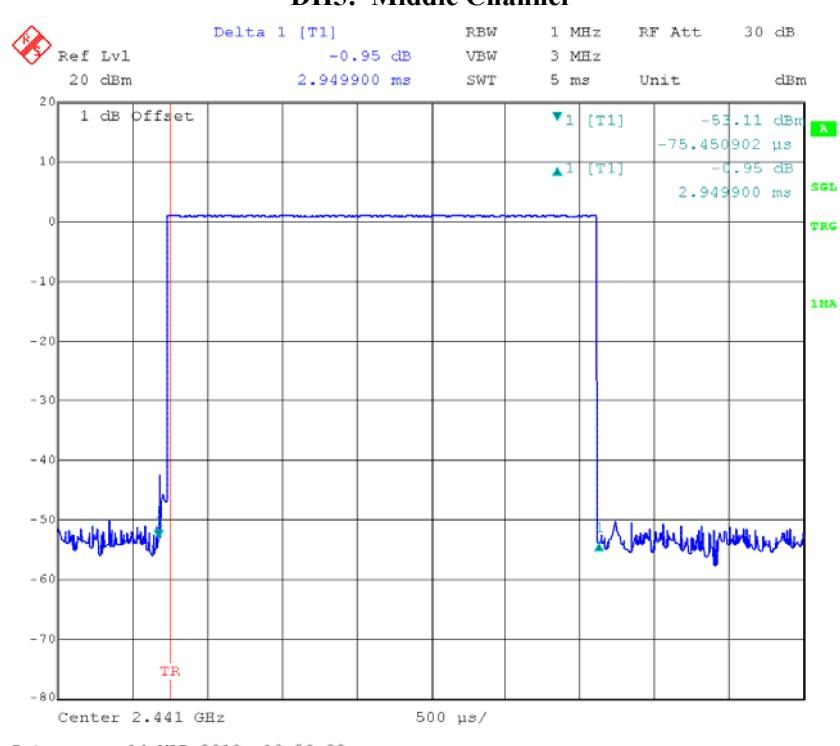
*EDR Mode ( $\pi/4$ -DQPSK):***2DH1: Middle Channel**
