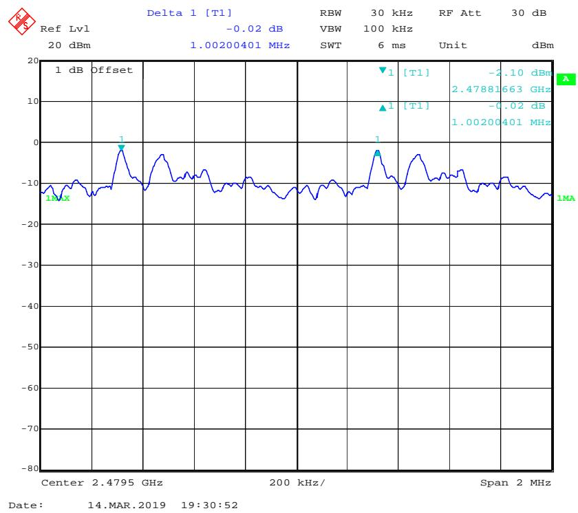
**FCC §15.247(a) (1) – 20 dB BANDWIDTH TESTING****Applicable Standard**
