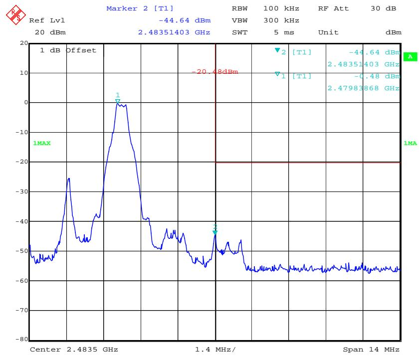
*EDR Mode ( $\pi/4$ -DQPSK):***Band Edge, Left Side**
