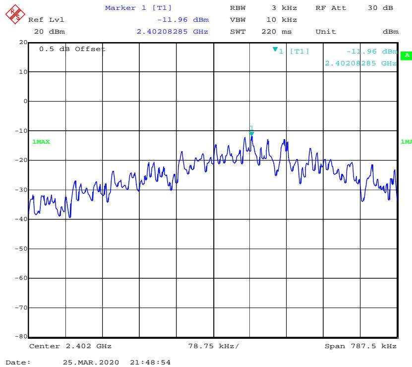
**Power Spectral Density, Middle Channel**
