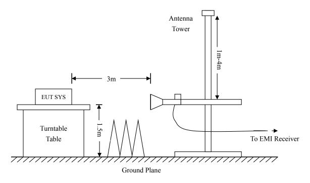
Frequency:9kHz-30MHz Frequency:30MHz-1GHz Frequency: Above 1GHz RBW=10KHz, RBW=120KHz, RBW=1MHz, VBW = 30KHzVBW=300KHz VBW=3MHz(Peak), 10Hz(AV) Sweep time= Auto Sweep time= Auto Sweep time= Auto Trace = max hold Trace = max hold Trace = max hold Detector function = peak Detector function = peak, QP Detector function = peak, AV
