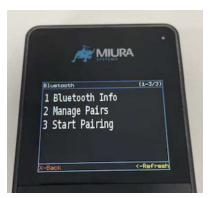
Option 1 *Bluetooth Info* will display the Name of the terminal and the Mac address. Option 2 *Manage Pairs* here you will see smart devices already paired to your terminal. Option 3 *Start Paring* this will put your terminal into the *Ready To Pair* mode where the Bluetooth Icon starts to flash.
