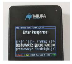
The Miura device keypad uses a basic scrolling function to allow the user to select the appropriate password character.
