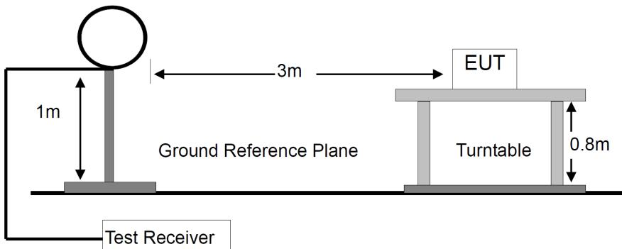
For Radiated Emission 30-1000MHz
