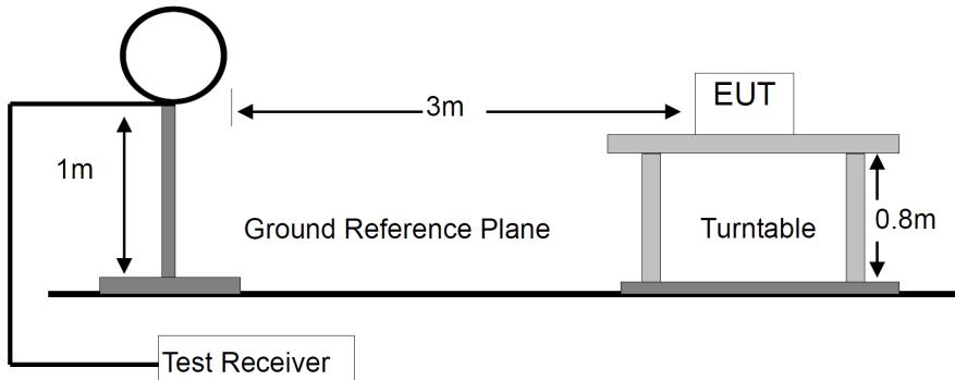
For Radiated Emission 30-1000MHz
