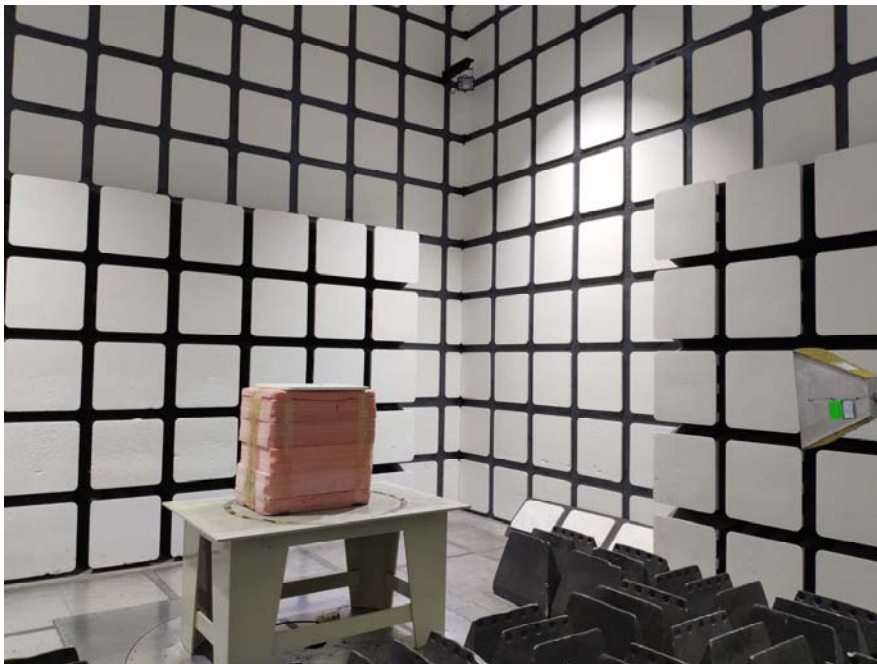
Radiated Emissions View (Above 1 GHz)
