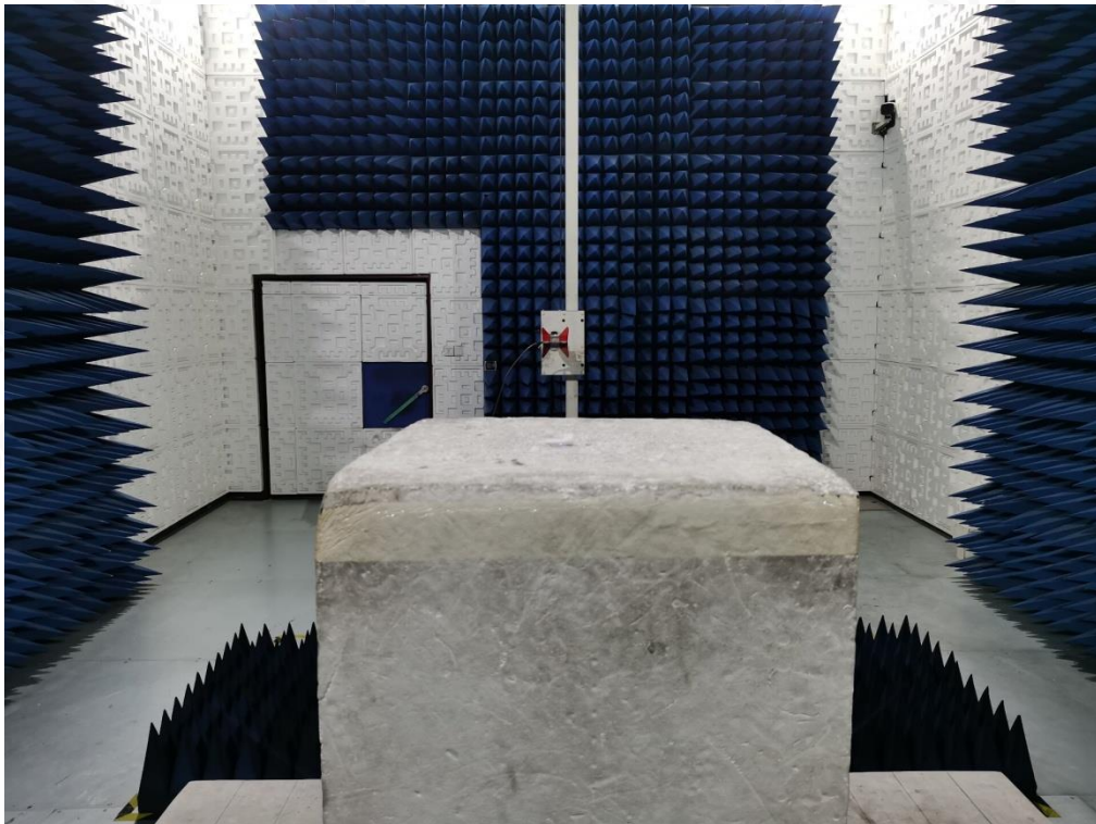
RADIATED EMISSION TEST SETUP ABOVE 1GHZ
