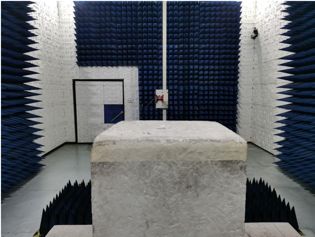
RADIATED EMISSION TEST SETUP ABOVE 1GHz
