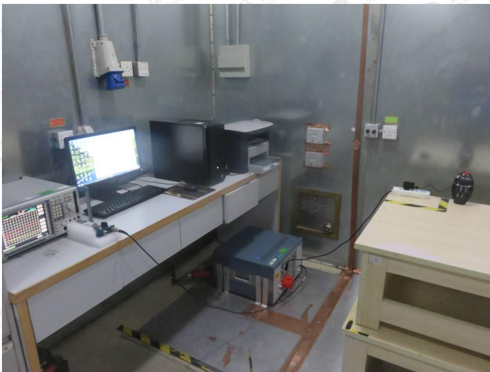
FCC RADIATED EMISSION TEST SETUP
