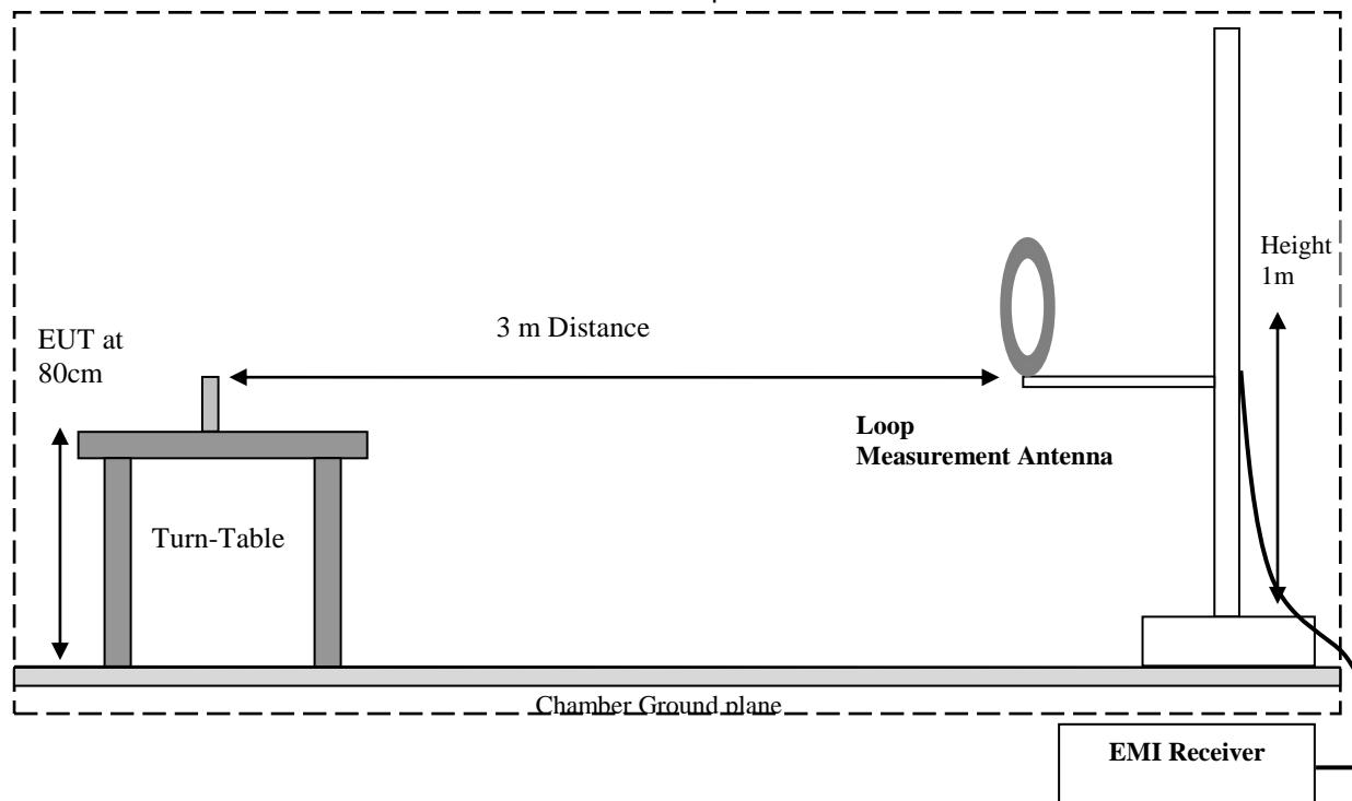
**Radiated Emissions Test Setup 30MHz-1GHz Measurements**
