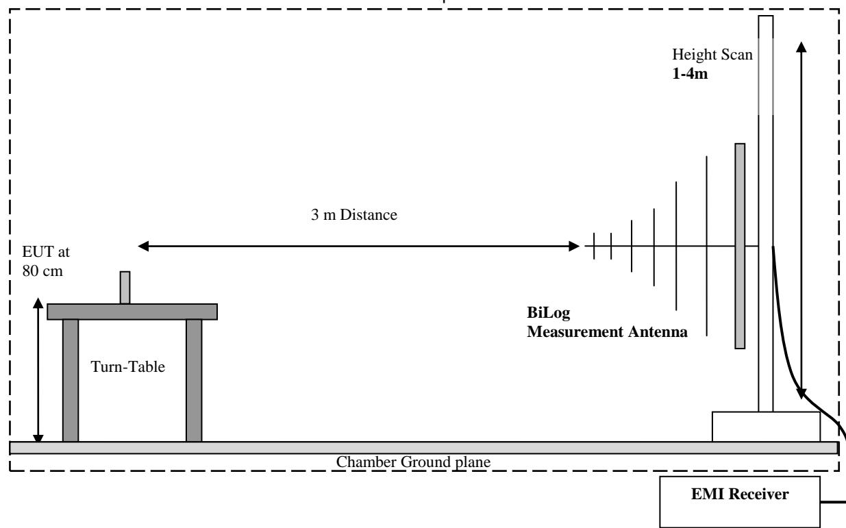
**Radiated Emissions Test Setup above 1GHz Measurements**
