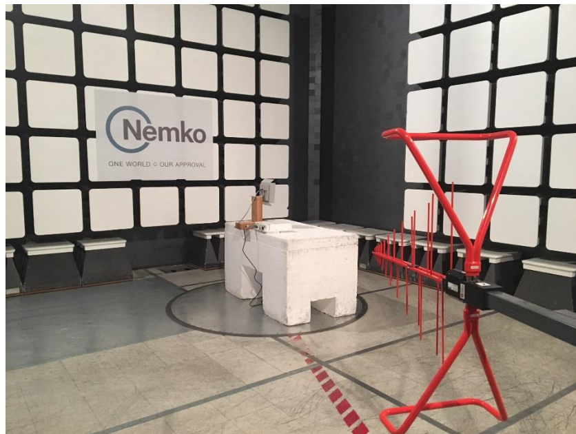
Figure 1.1-2: Radiated emissions setup photo – below 1 GHz
