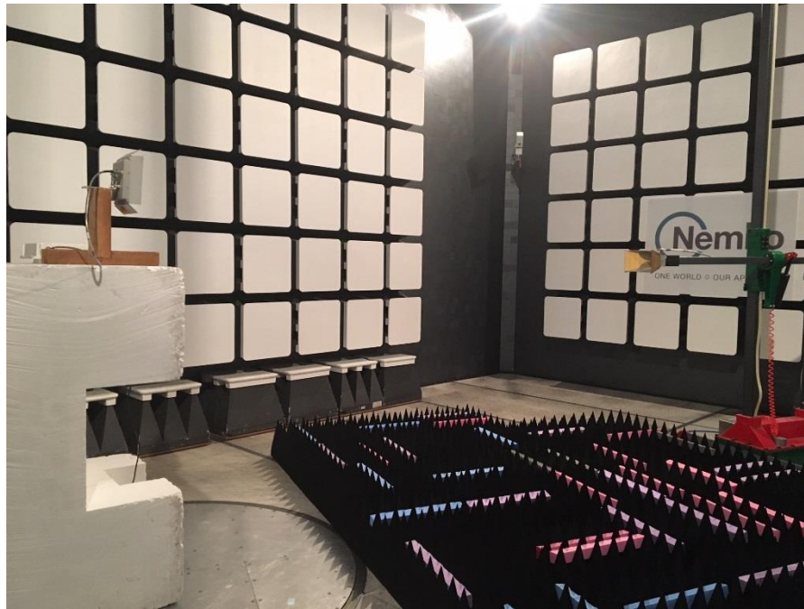
Figure 1.1-3: Radiated emissions setup photo – above 1 GHz
