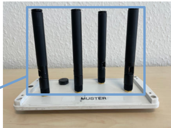
4x HG2458RD-RSP Antenna - 433.05-434.79 MHz - 902-928 MHz - 2280-2600 MHz - 5780-5875 MHz (Broadband Receiver)
