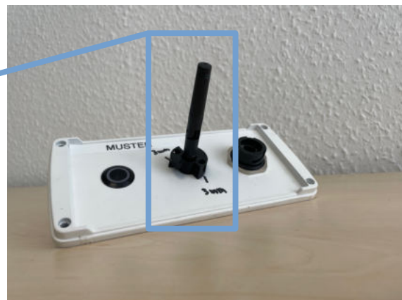
1x 2JW035-C442B Antenna - 2412-2472 MHz - 5180-5825 MHz (WiFi Receiver)
