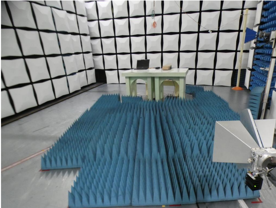
Photo 3: Test setup for radiated measurements (computer peripheral setup, 1 GHz – 18 GHz; unintentional radiator §15.109, ANSI C63.4)
