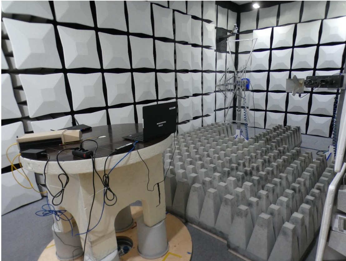
Photo 4: Test setup for radiated measurements (computer peripheral setup, 18 - 26 GHz; unintentional radiator §15.109, ANSI C63.4)
