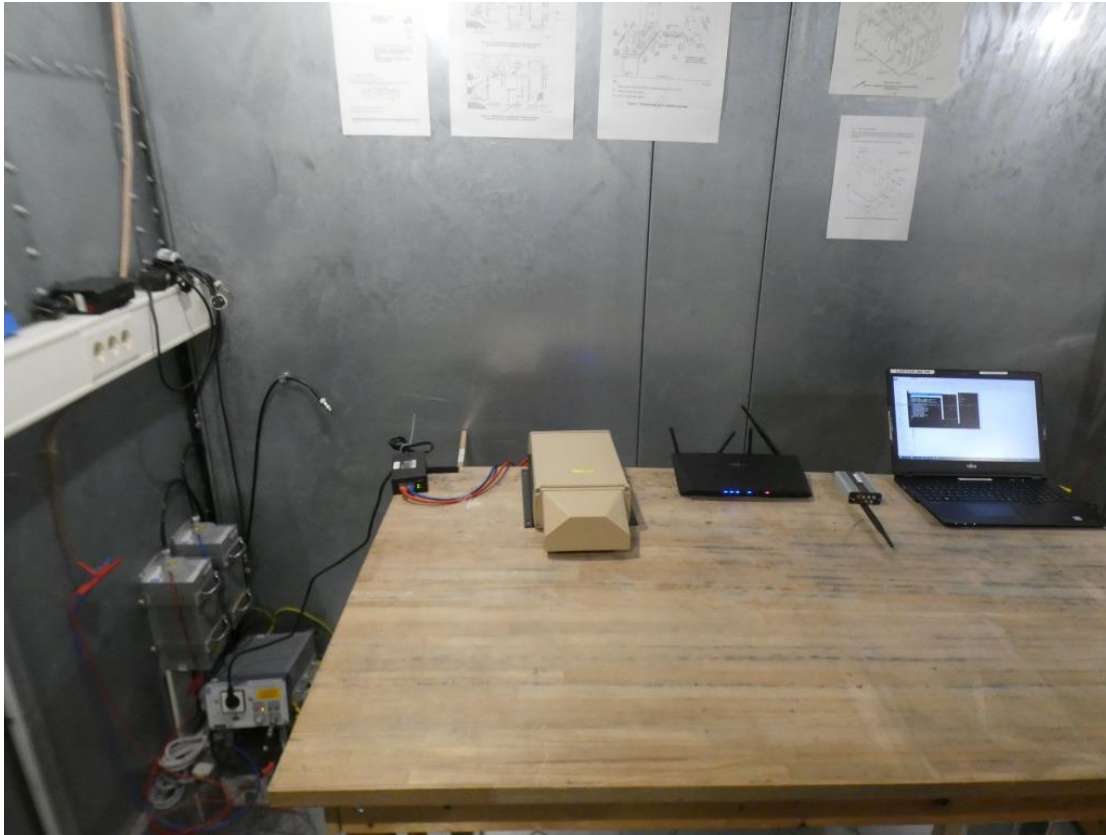
Photo 1: Test setup for conducted measurements (Test Setup: computer peripheral setup, AC mains connection: connected via auxiliary equipment, unintentional radiator §15.107, ANSI C63.4)
