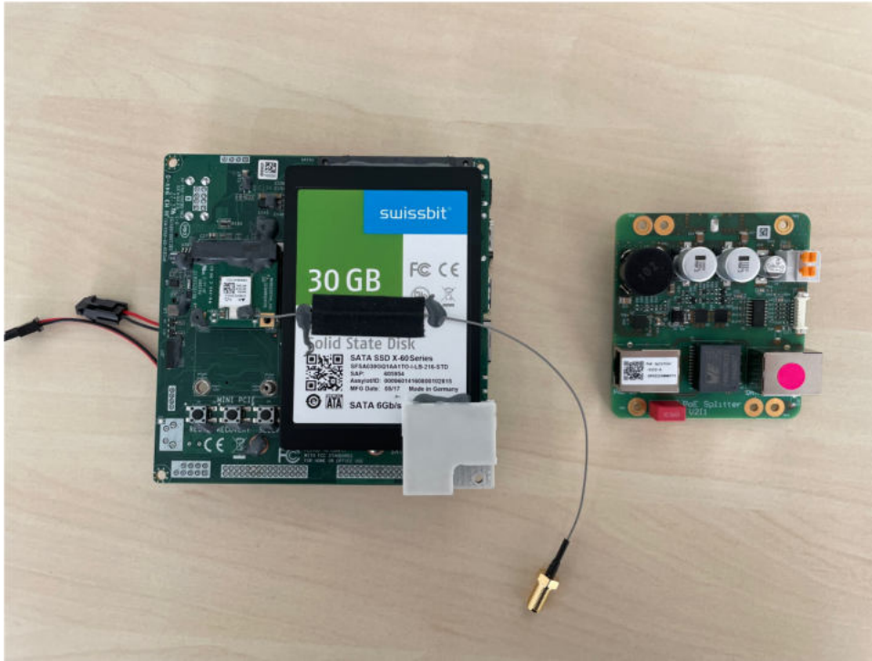
Main board with Nvidia TX2 SOM, SSD and WiFimodule / PoE splitter
