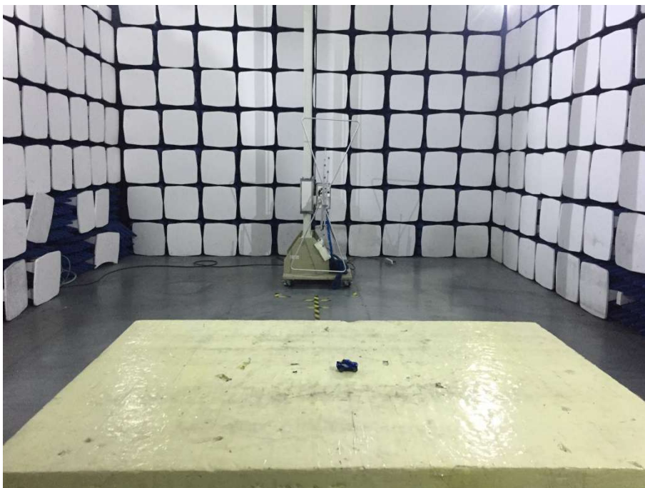
Radiated Emission Test Setup (from 30 MHz to 1 GHz) from 0.8M-Height Turntable Test Table
