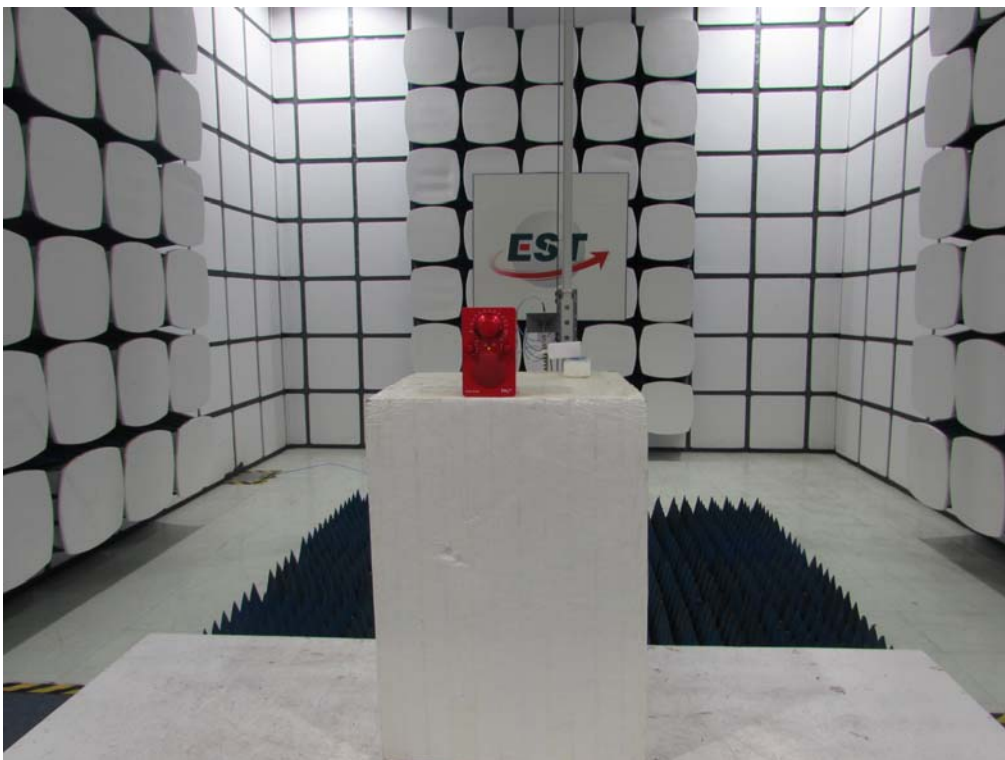
Radiated Test (1000-25000 MHz)
