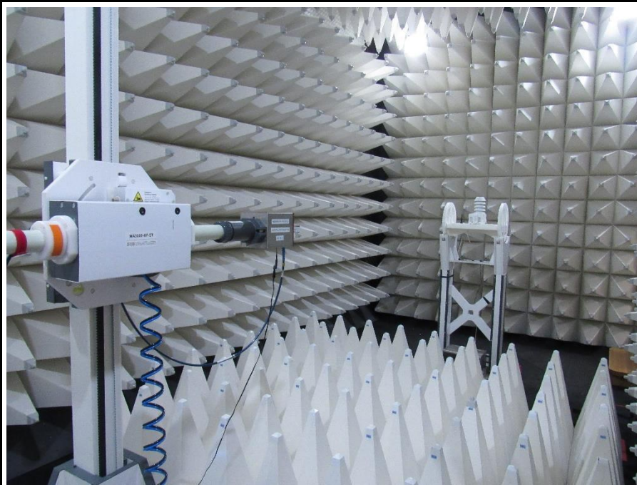
Setup for measurements above 1 GHz
