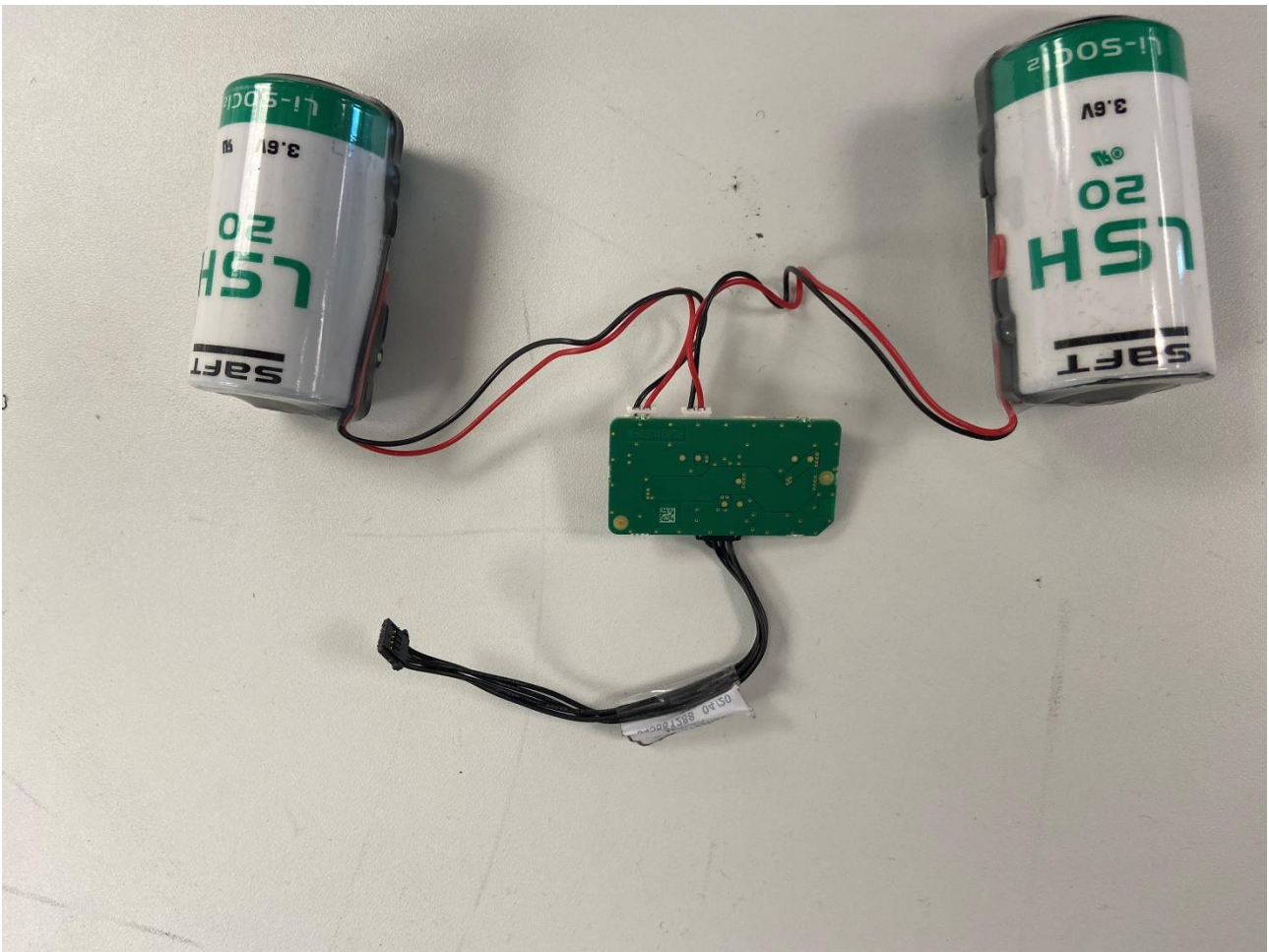
Photo 20. IOTPW and batteries, back view
