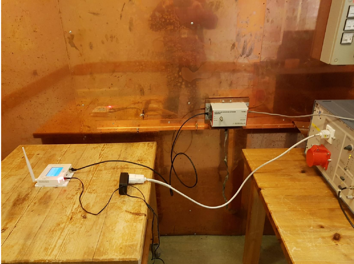
Test set up Conducted emission 150 kHz – 30 MHz
