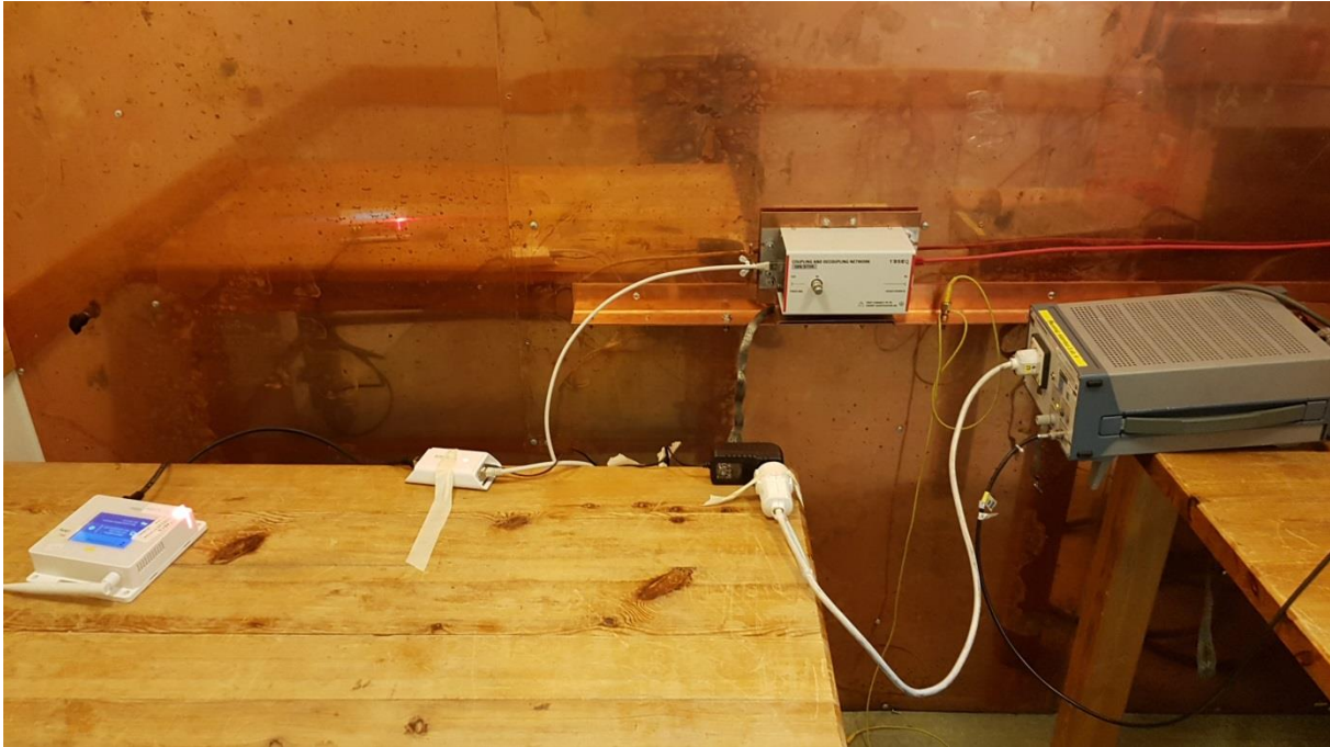
Photo of the test set-up for conducted emission with PoE injector
