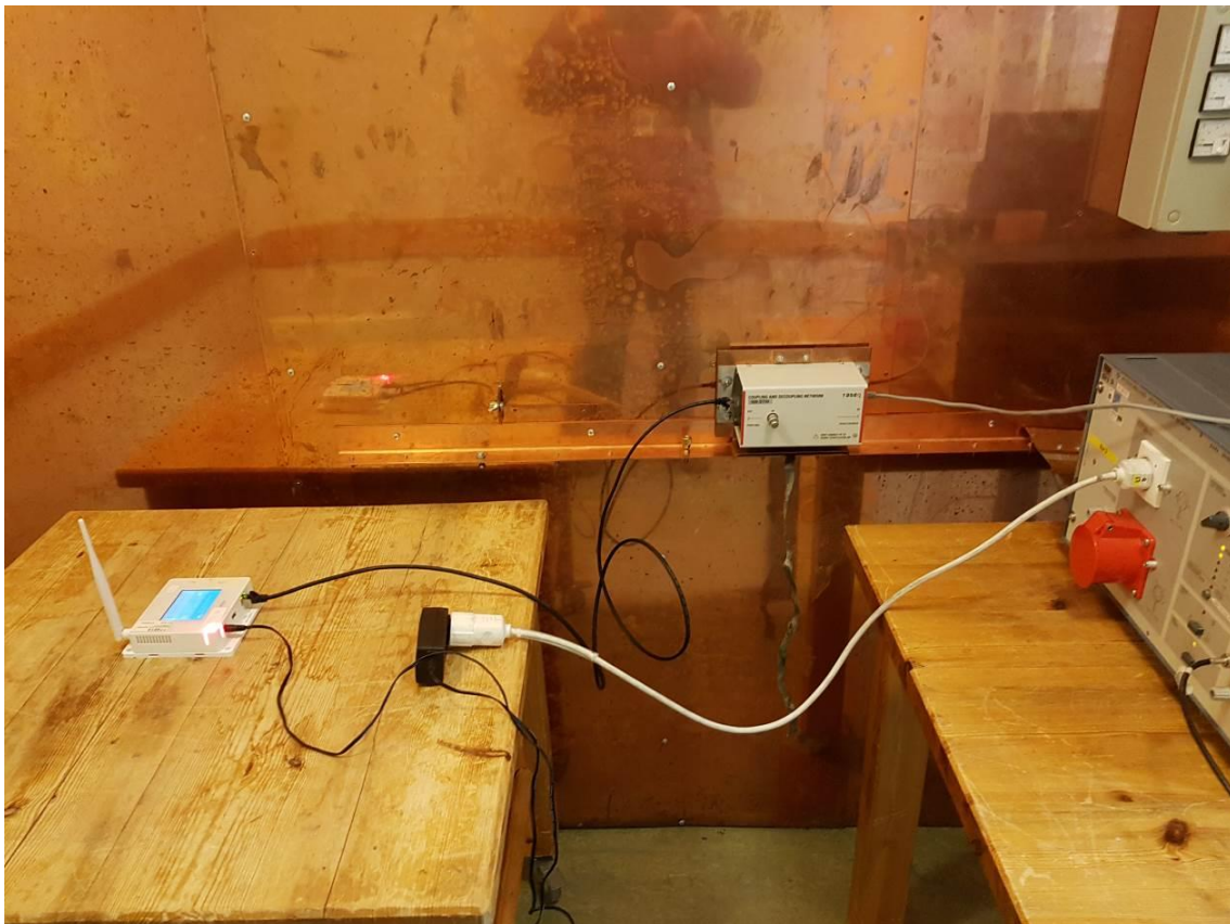
Photo of the test set-up for conducted emission AC DC adapter
