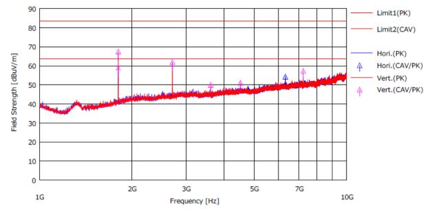
Test mode : 1 GHz ~ 10 GHz ( Worst case : GFSK\_Lowest Frequency )
