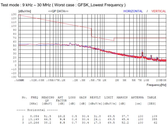
4.4.7.7 Measurement Plot\_Radiated Spurious Emissions
