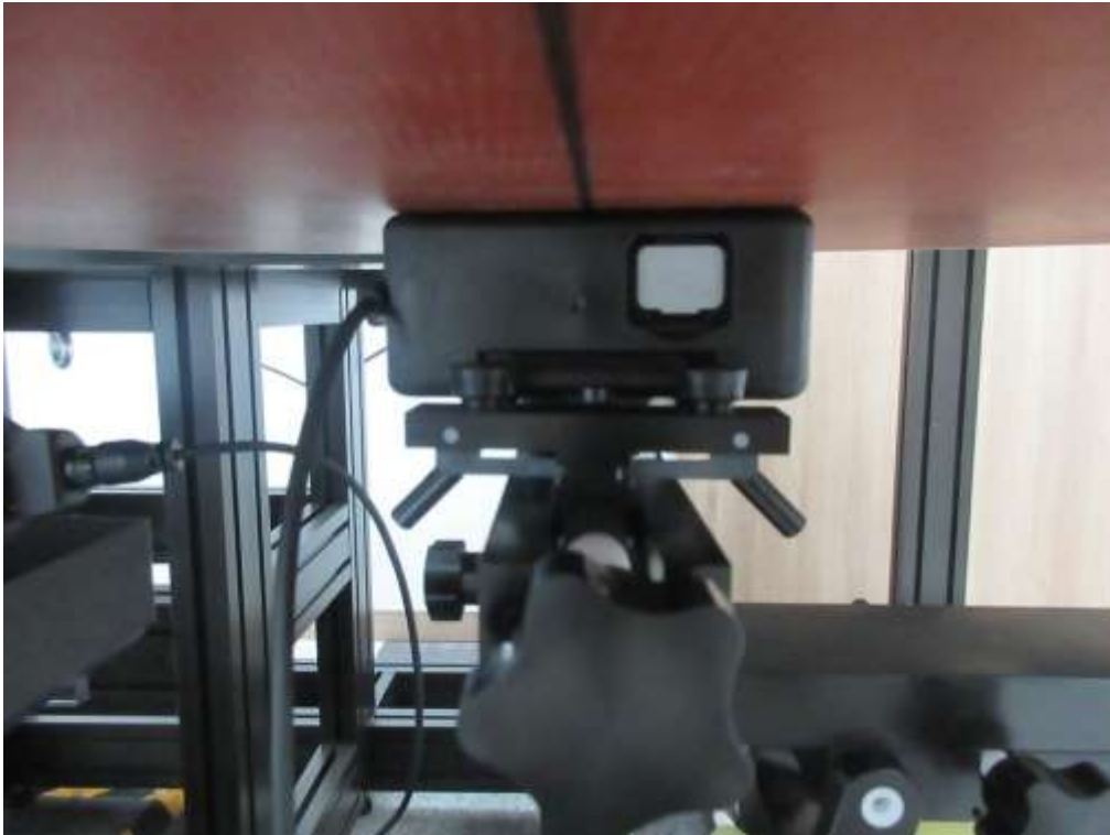
Front from Flat Phantom (Separation Distance: 0 cm) – Silicon case with Headset
