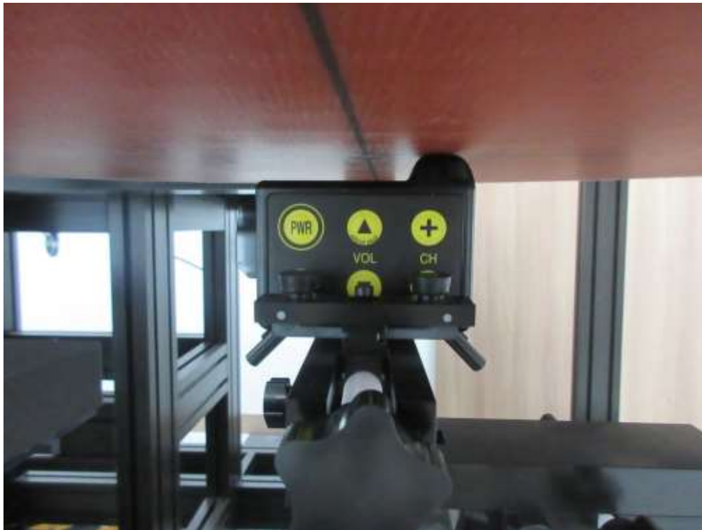
Top from Flat Phantom (Separation Distance: 0 cm)
