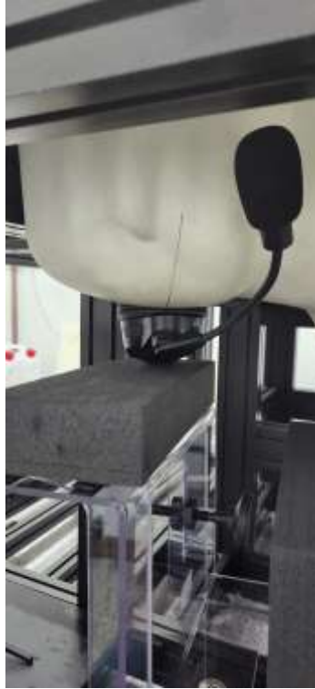
Right Ear from SAM Phantom (Separation Distance: 0 cm)
