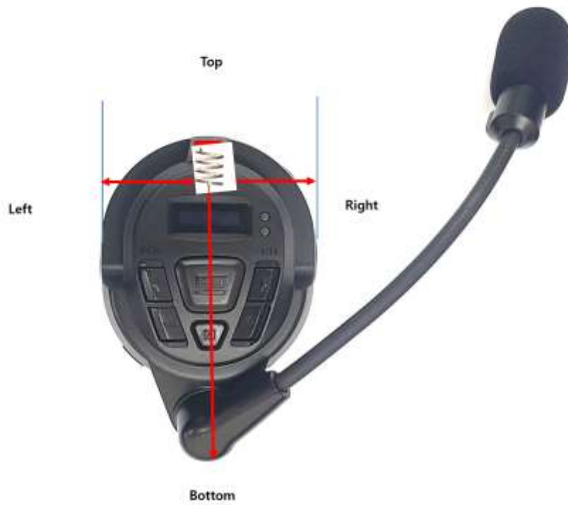
Figure F-1 Antenna Location
