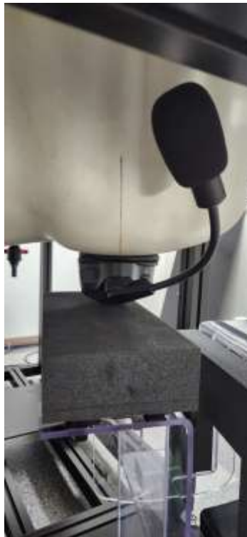
Left Ear from SAM Phantom (Separation Distance: 0 cm)
