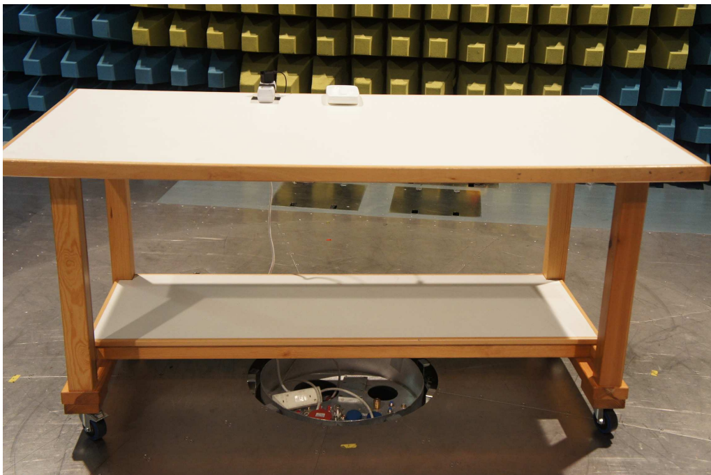
Picture 6: SAC, radiated emission test 30 MHz – 1 GHz – Standby (rear view)
