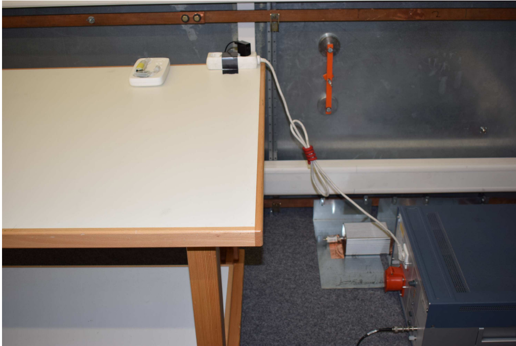
Picture 11: AC power line conducted emission – Charging (front view)
