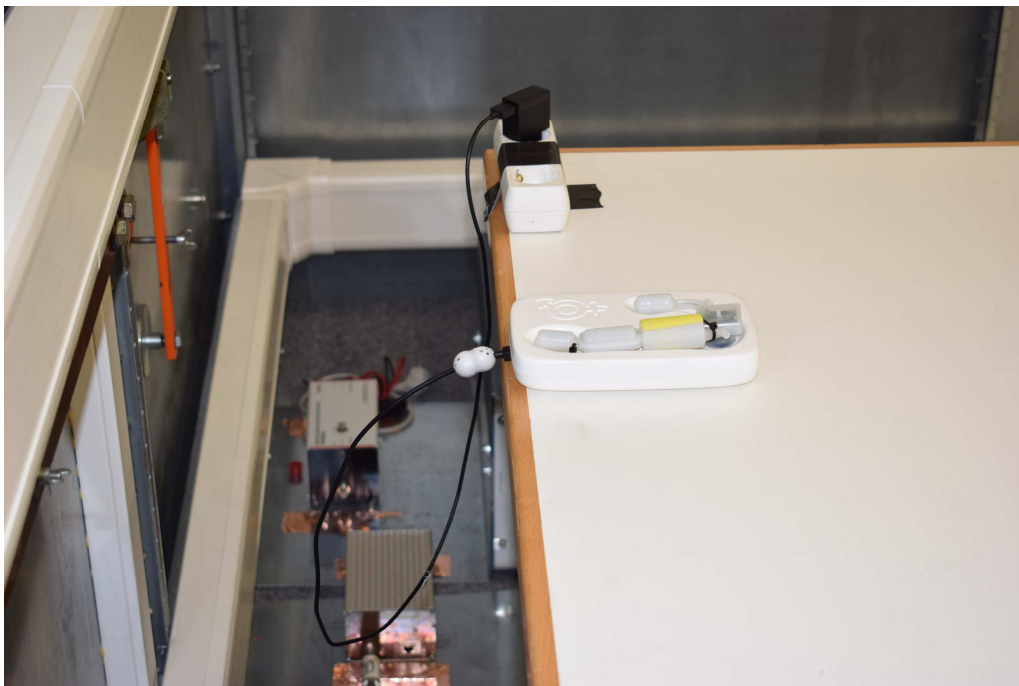
Picture 12: AC power line conducted emission – Charging (rear view)
