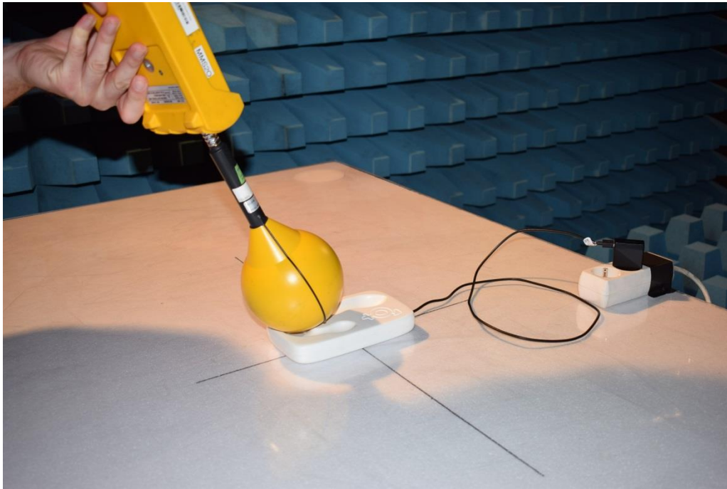
Picture 7: Setup of magnetic field test for standby mode
