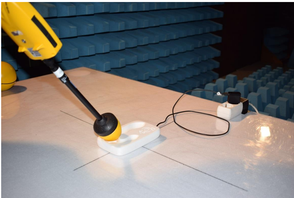
Picture 8: Setup of electric field test for standby mode
