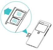
Remove the SD Card tray from the ChecOut M device. When reinserting the SD card, ensure that it is in the proper orientation relative to the tray.
