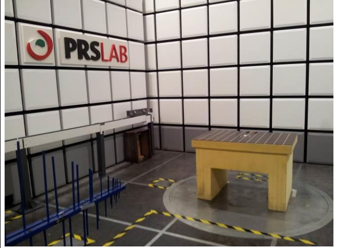
PHOTO N°2 SETUP FOR RADIATED MEASUREMENT <1GHz
