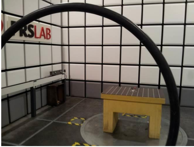
PHOTO N°2 SETUP FOR RADIATED MEASUREMENT <1GHz
