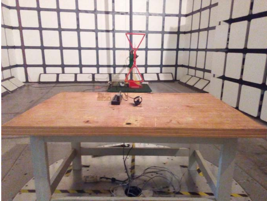
Radiated Emissions View (Below 1 GHz)
