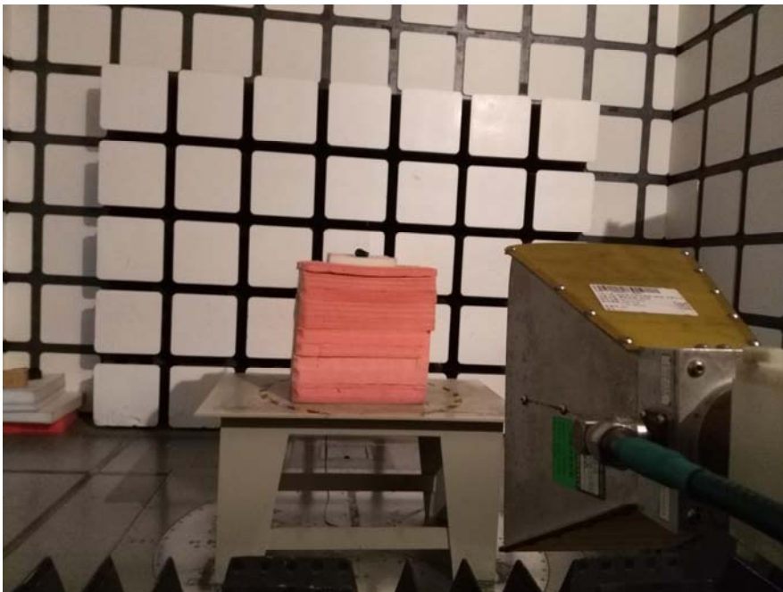
Radiated Emissions View (Above 1 GHz)
