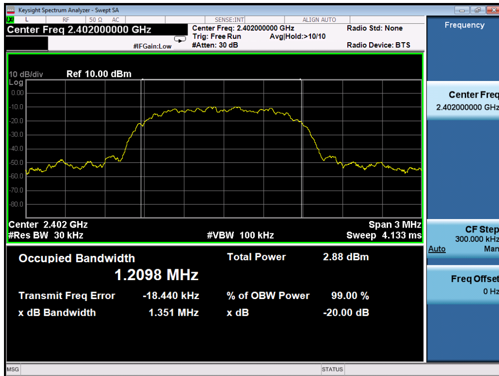
TEST PLOT OF BANDWIDTH FOR LOW CHANNEL
