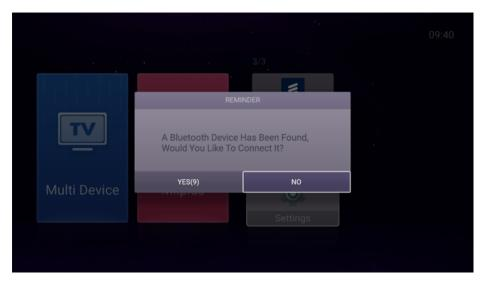
3. When indicating the reminder, the device will pair with the new Bluetooth remote controller automatically if no operation occurs within ten seconds.
