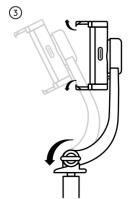
Adjust the arm of the selfie stick to the desired position, if the arm is hard to move, loosen the screw. Tighten the
