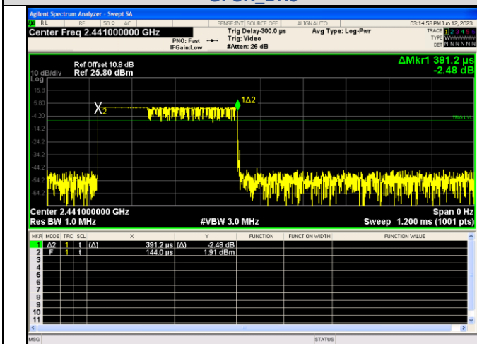
Pulse Width \pi /4DQPSK_2-DH1
