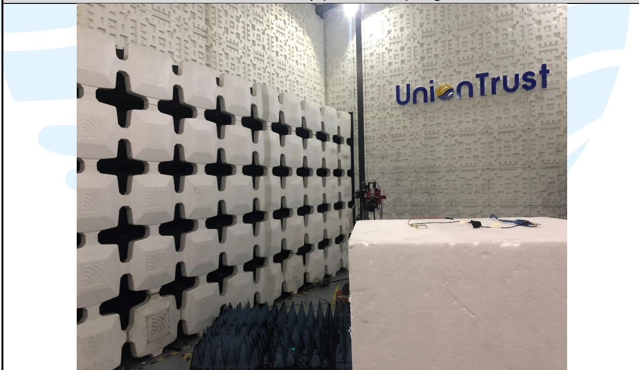
Radiated emission Test Setup (Above 1 GHz) –Right Earbuds
