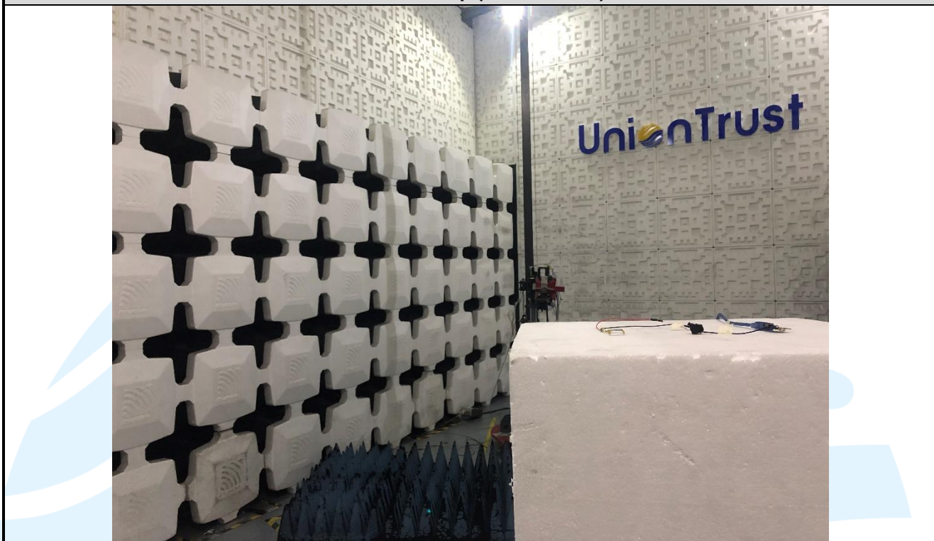
Radiated emission Test Setup (Above 1 GHz) –Left Earbuds
