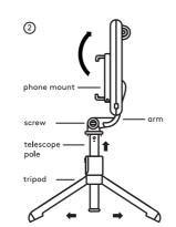
To use the tripod, pull the telescope pole up and open the legs of the tripod, and place it on a sturdy flat surface.
