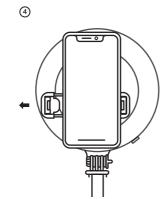
Rotate the phone mount, pull the arm of the phone mount open, and place your phone into it. The mount rotates so you can stream in either landscape or portrait settings. Close the legs of the tripod to use it as a selfie stick
