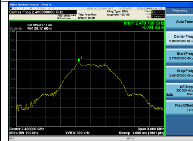
GFSK on Channel 39
