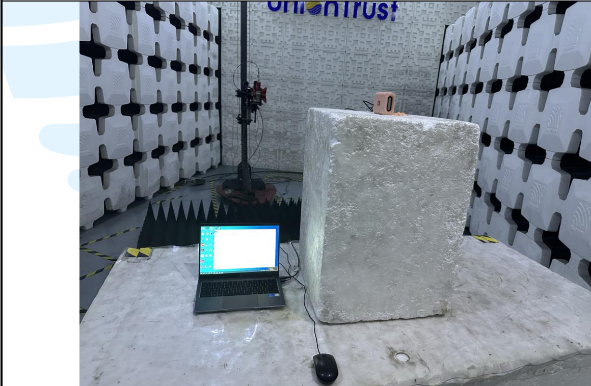
Radiated emission Test Setup (Above 1 GHz)
