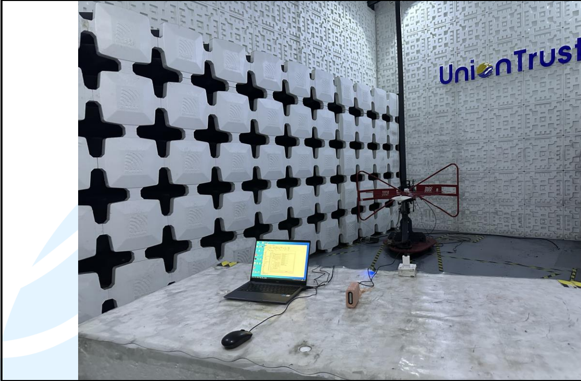
Radiated emission Test Setup (30 MHz~1 GHz)
