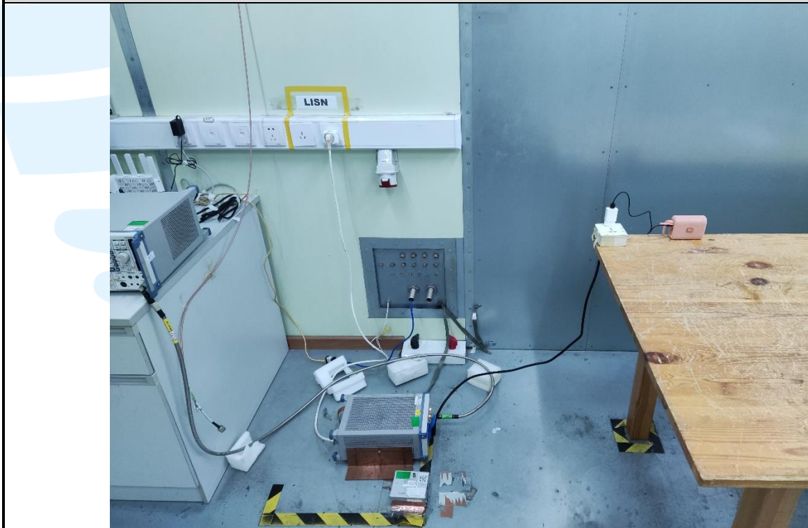
Conducted Emission Test Setup
