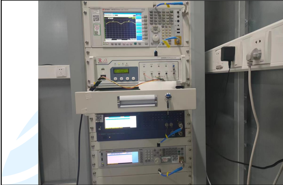
RF Conducted Test Setup
