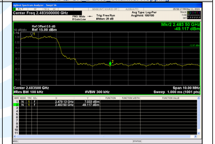
Out Of Band Emission(Right) π/4DQPSK 2-DH5 Channel Hopping
