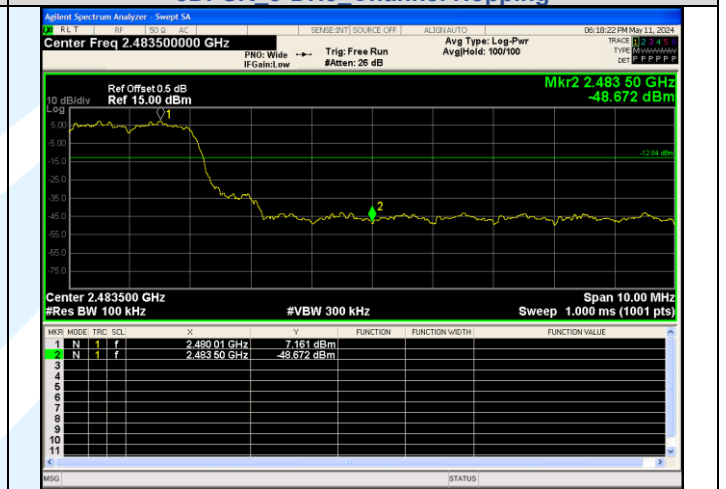
Out Of Band Emission(Right) 8DPSK 3-DH5 Channel Hopping
