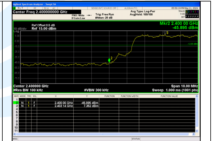
Out Of Band Emission(Left) \pi/4 DQPSK 2-DH5 Channel Hopping
