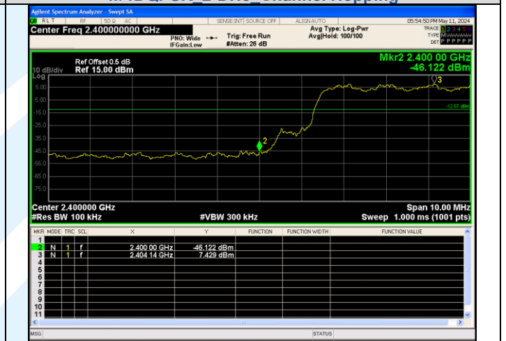
Out Of Band Emission(Left) π/4DQPSK 2-DH5 Channel Hopping
