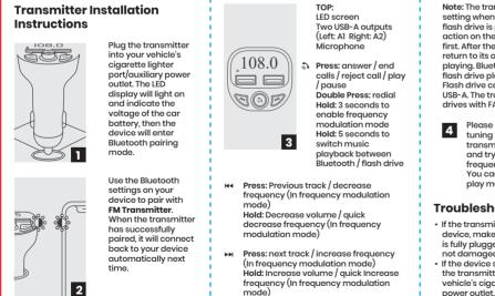
Note: The transmitter will recall the last setting when turned back on. When the flash drive is playing, if there is an audio action on the mobile, it will be executed first. After the response is completed, it will return to its original state and continue playing. Bluetooth priority is higher than flash drive playback. Flash drive can only use the A2 port of USB-A. The transmitter only supports flash drives with FAT32 format
