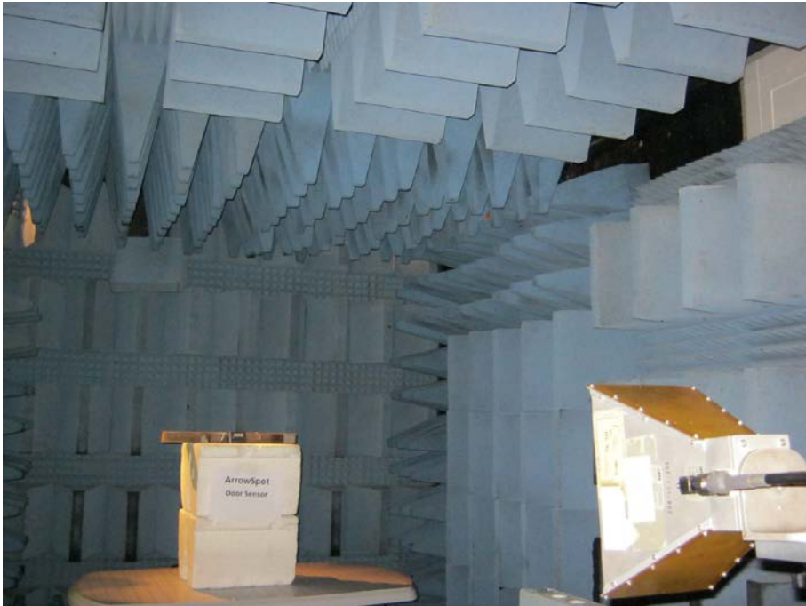
Radiated Emission Test 1.0-5.0GHz
