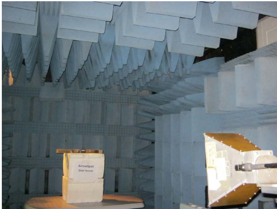
Figure 5. Radiated Emission Test 1.0-5.0GHz
