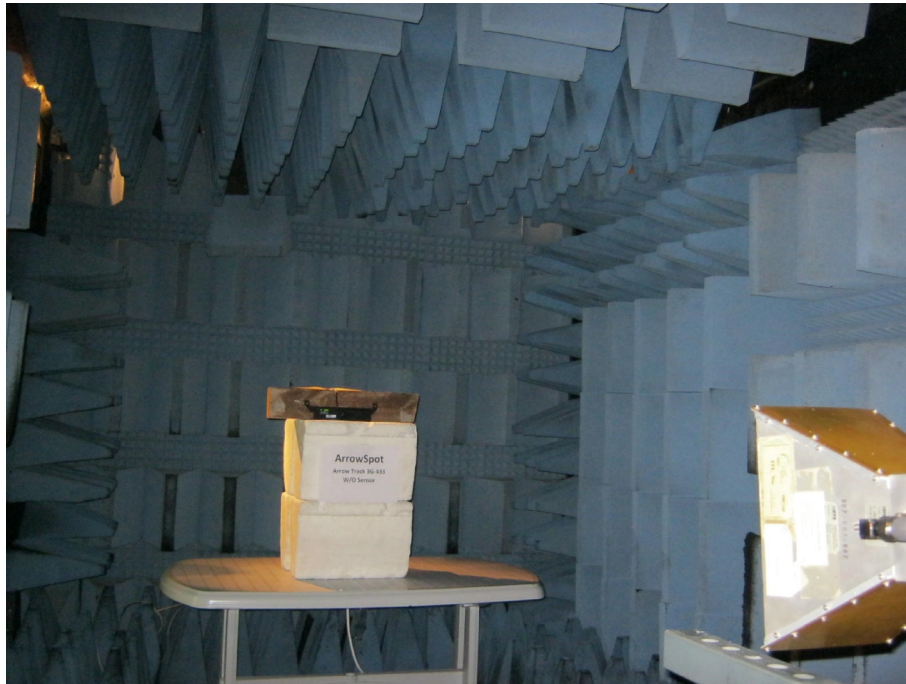
Figure 6. Radiated Emission Test 1.0-5.0GHz
