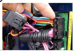
Connect controller male connector to ArrowTrack female
