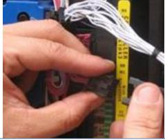
Take out the green RMM power connector and replace it with ArrowTrack connector
