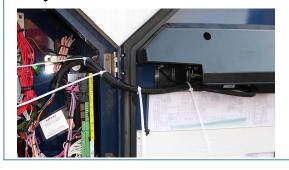
If there is RMM: Take out the green RMM power connector and replace it with ArrowTrack connector
