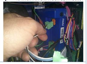
Connect RMM connector to ArrowTrack wire (male with female)
