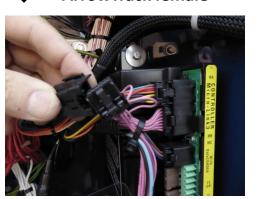
Take the green power 24AC connector and connect it with ArrowTrack connector
